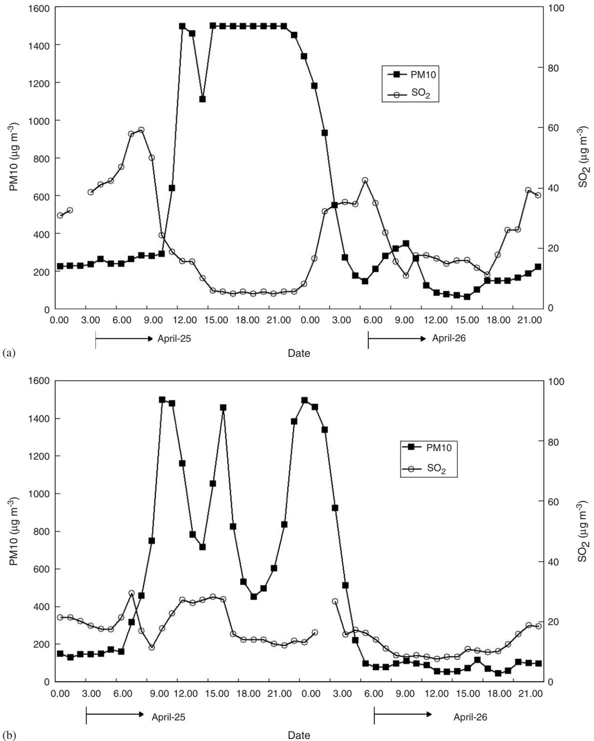
Fig. 2. The 1-h  $\text{SO}_2$  and  $\text{PM}_{10}$  concentrations during the two dust events: (a) 6–7 April and (b) 25–26 April. The  $\text{PM}_{10}$  concentrations appear to be saturated at  $1500 \mu\text{g m}^{-3}$  but the actual number may have been much higher because the “analog output” used in TEOM online data acquisition was set to full scale at  $1500 \mu\text{g m}^{-3}$ .
