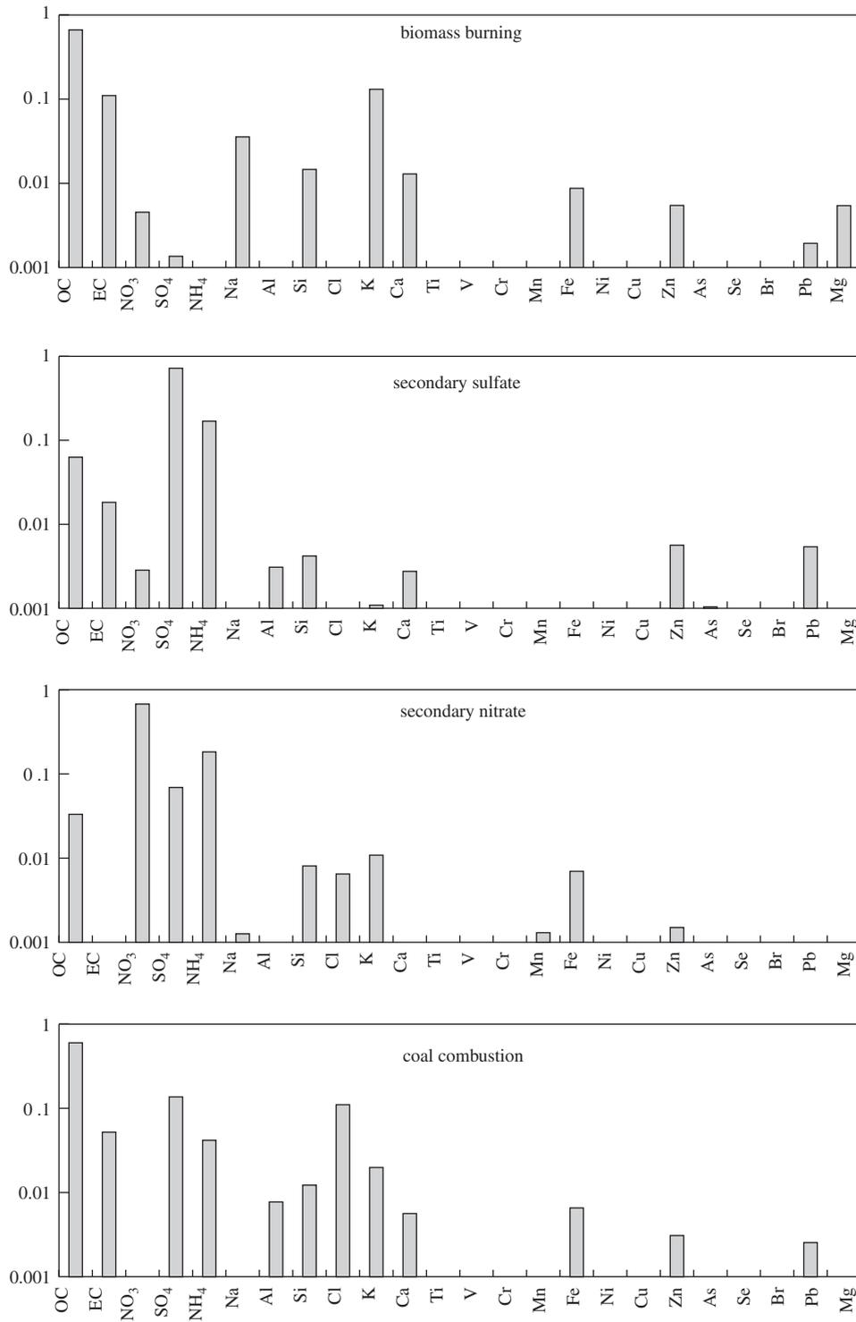
Fig. 5. Sources profiles resolved from PM<sub>2.5</sub> samples for biomass burning, secondary sulfates, secondary nitrates, coal combustion, industry, motor vehicles, yellow dust, and road dust.
