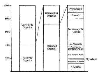
Figure 1. Mass balance for elutable organic matter contained in fine cigarette smoke particles.
